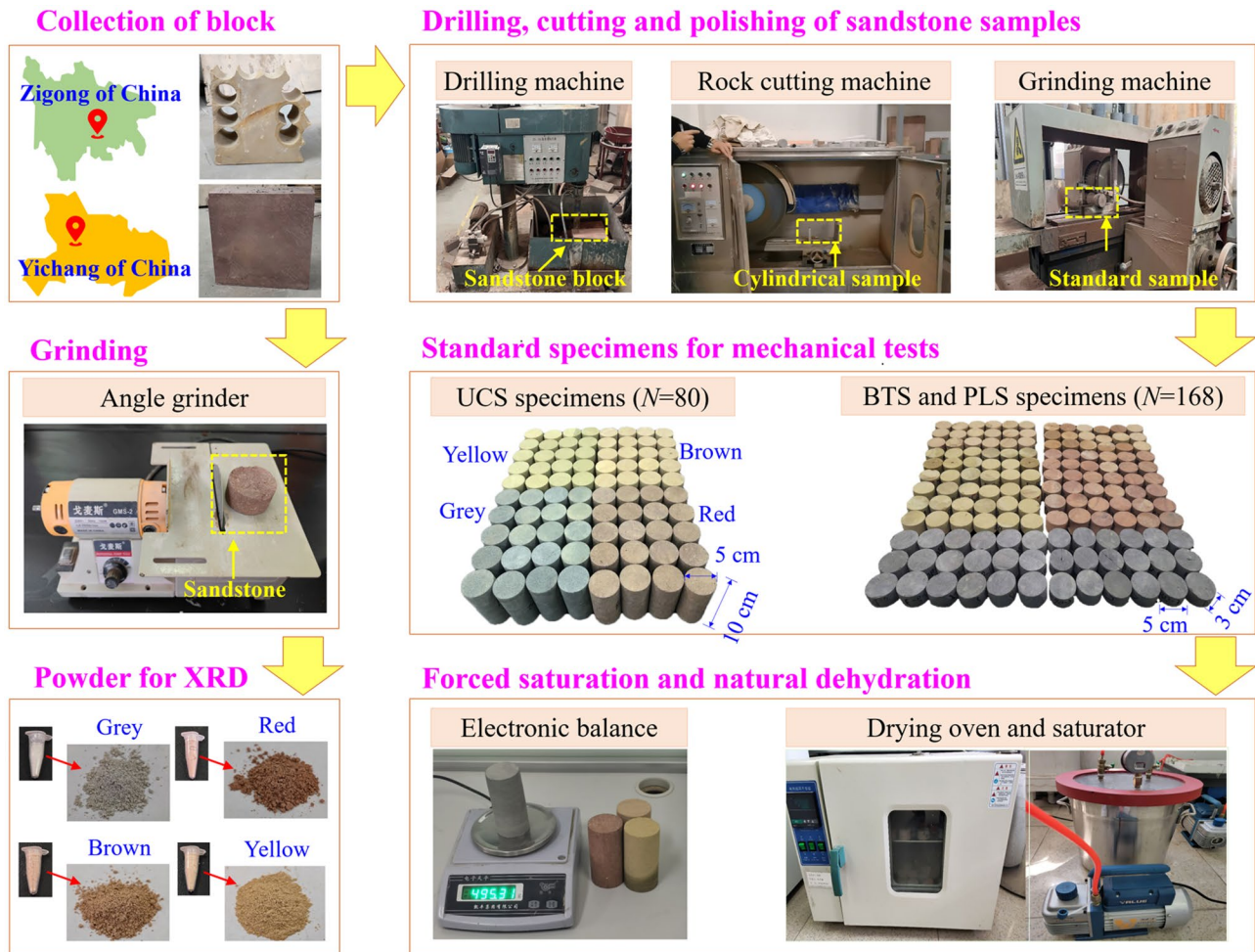
Fig. 1 Preparation procedure of cylindrical sandstone samples and powder
