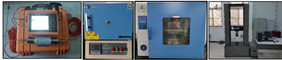
Fig. 4 a Ultrasonic p-wave speed detector. b KSL-1200X muffle furnace. c Electric blast drying oven. d Electro-hydraulic servo universal testing machine
