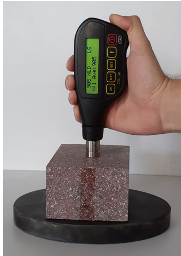
Fig. 5 Leeb hardness instrument applied in the experiments
