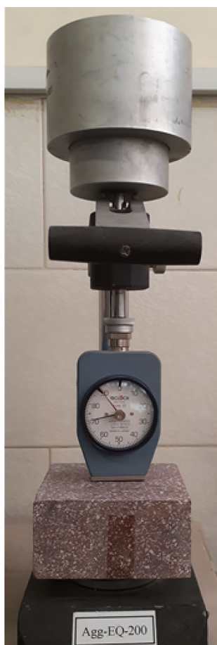
Fig. 7 Applied D-type Shore hardness testing instrument
