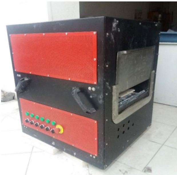
Fig. 1 The 6 kW microwave oven used in the tests
