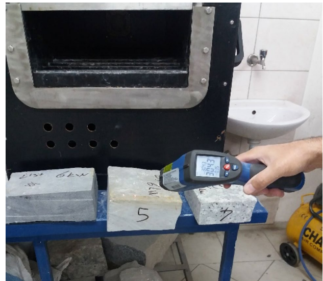
Fig. 2 The measurement of the surface temperatures
