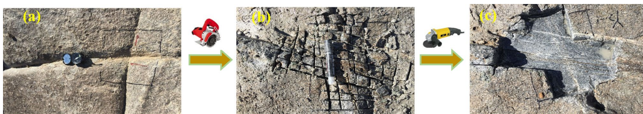
Fig. 3 Exposure of fresh fracture surface by removing the influence range of surface weathering in research area. (a) Weathered fracture surface. (b) Process of removing the weathered fracture surface using cutting machine. (c) Exposed fresh fracture surface using grinder machine
