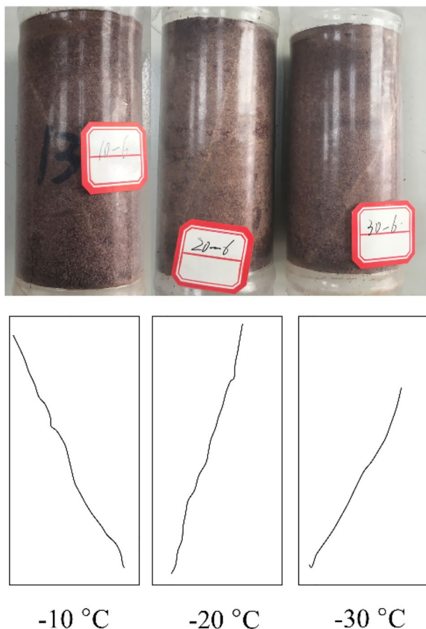
Fig. 4 Failure morphology of sandstone at different temperatures (the confining pressure is 6 MPa)
