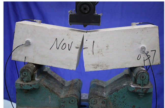
Fig. 4 Three-point bending tests
