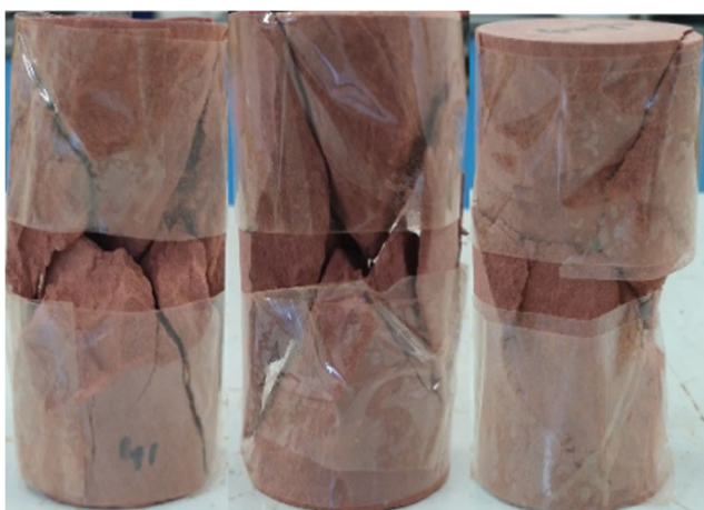
Fig. 17 Failure modes of the three samples in the test group with 70% initial damage and 40 freeze–thaw cycles
