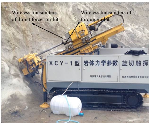
Fig. 1 Drilling process monitoring system (DPM)
