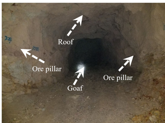
Fig. 12 Image of the goaf used in the stability monitoring experiment
