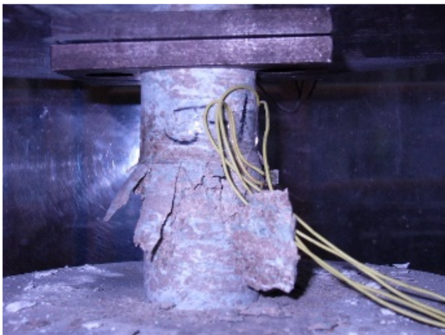
Fig. 5 Compression experiment of the bauxite rock mass
