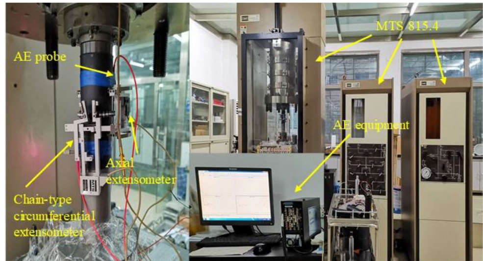
Fig. 2 Mechanical testing system and AE acquisition system
