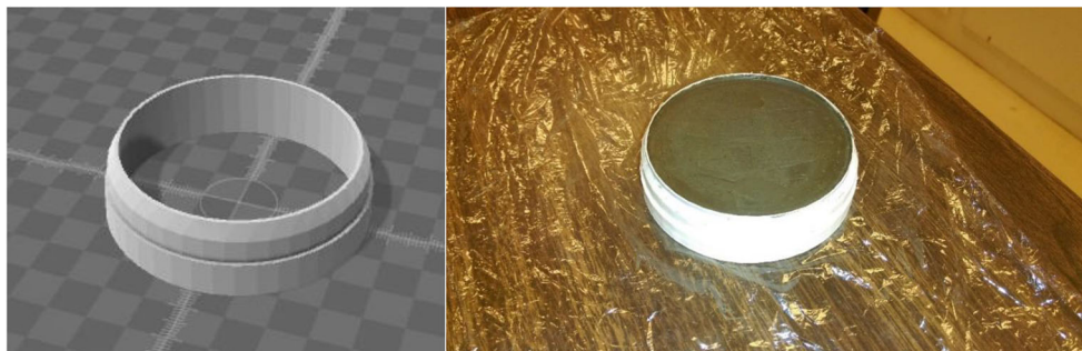
Fig. 1 3D model of custom sized ring (left) and soil sample inside 3D printed ring (right)
