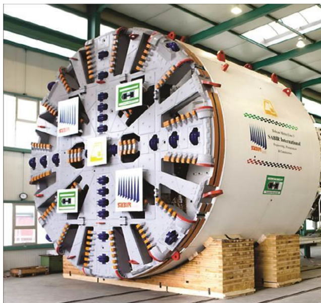
Fig. 10 TBM machine used in the excavation of SEL6 tunnel
