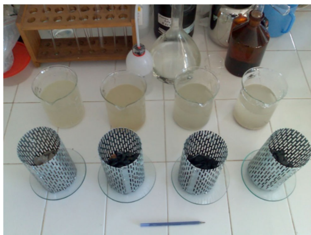
Fig. 3 An image of the salt crystallisation ( \text{MgSO}_4 ) test on aggregates
