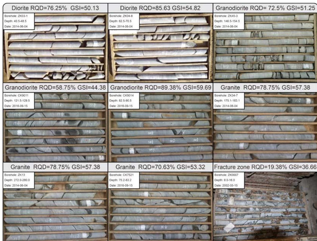
Fig. 5 Geological logging of drilling boreholes
