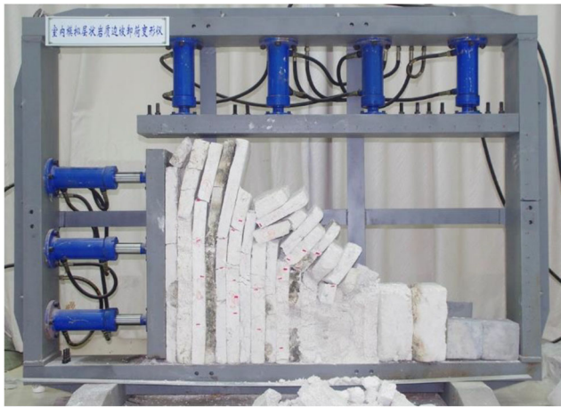
Fig. 7 The final failure stage
