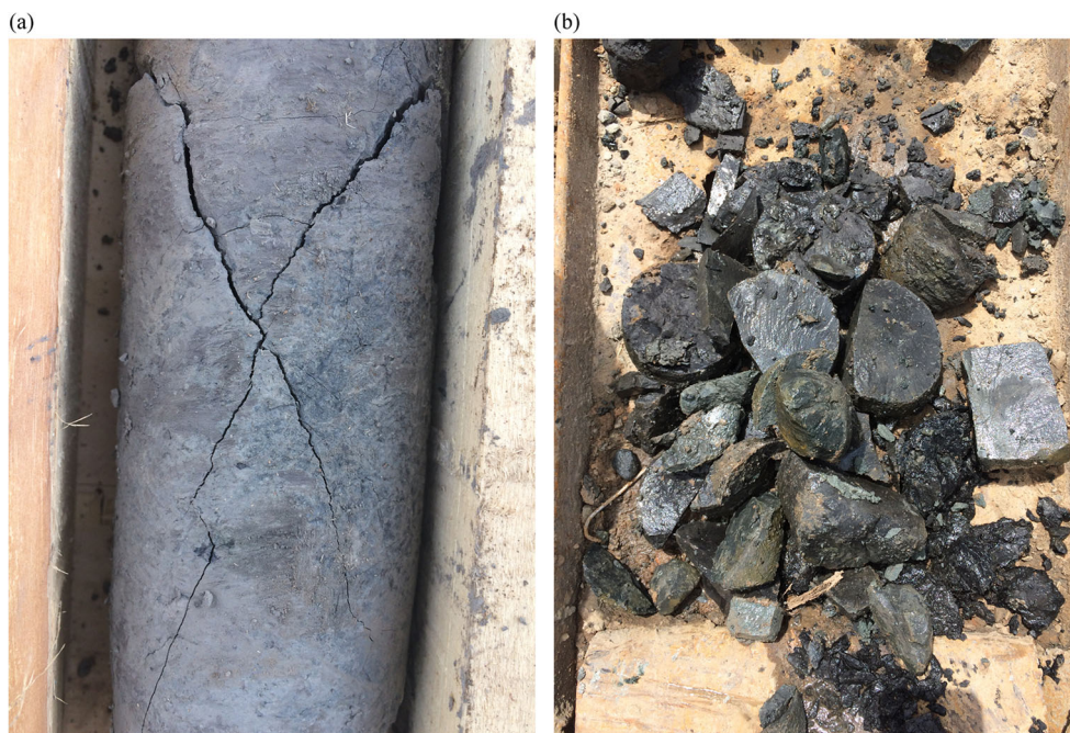
Fig. 10 Photos of borehole 2-SD2 showing vertical fractures developed in fractured zone (a) and cracked strata developed in caved zone (b)
