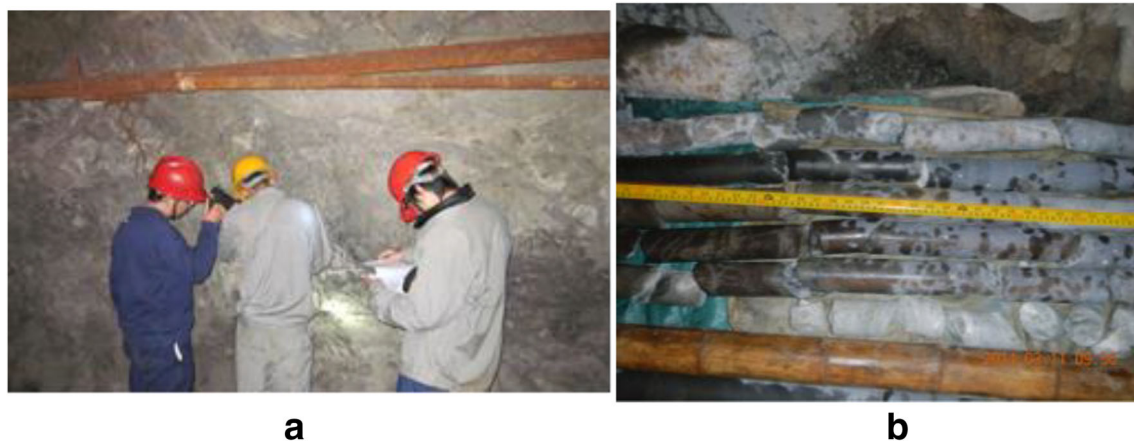
Fig. 30 Field investigation. a Joint mapping and b core drilling
