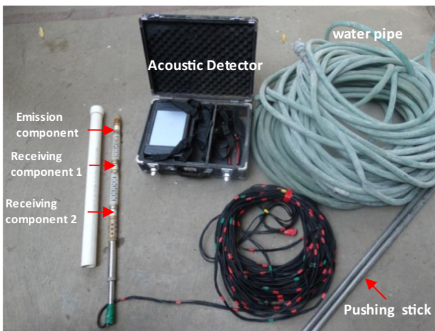
Fig. 9 The integrated ultrasonic wave detection equipment for rock damage
