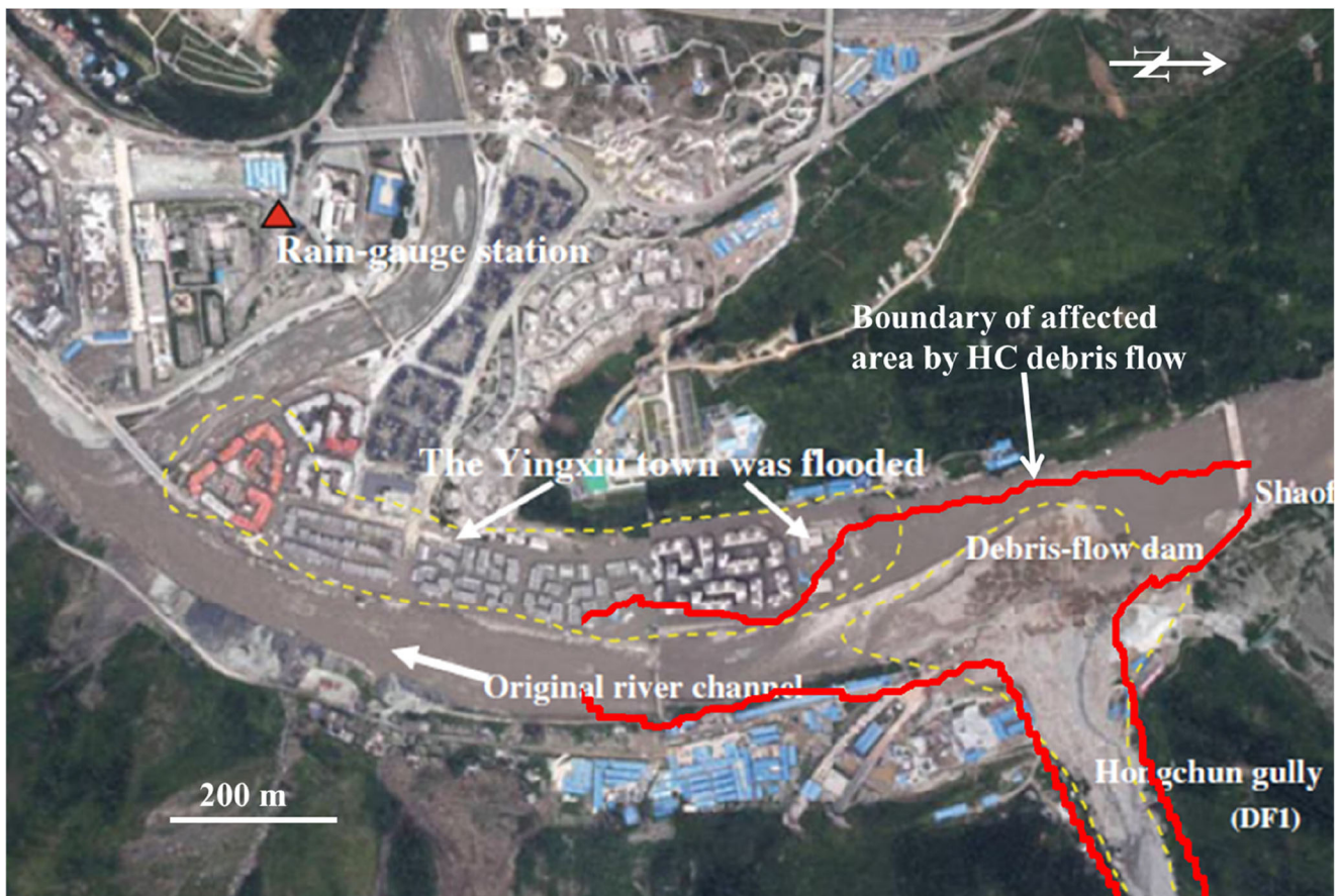
Fig. 12 The area affected by HC debris flow on the deposition zone. The base image is from Tang et al. (2011a, 2011b), an aerial photo taken on 15 August 2010 showing the HC debris flow fan, and the inundated area in
