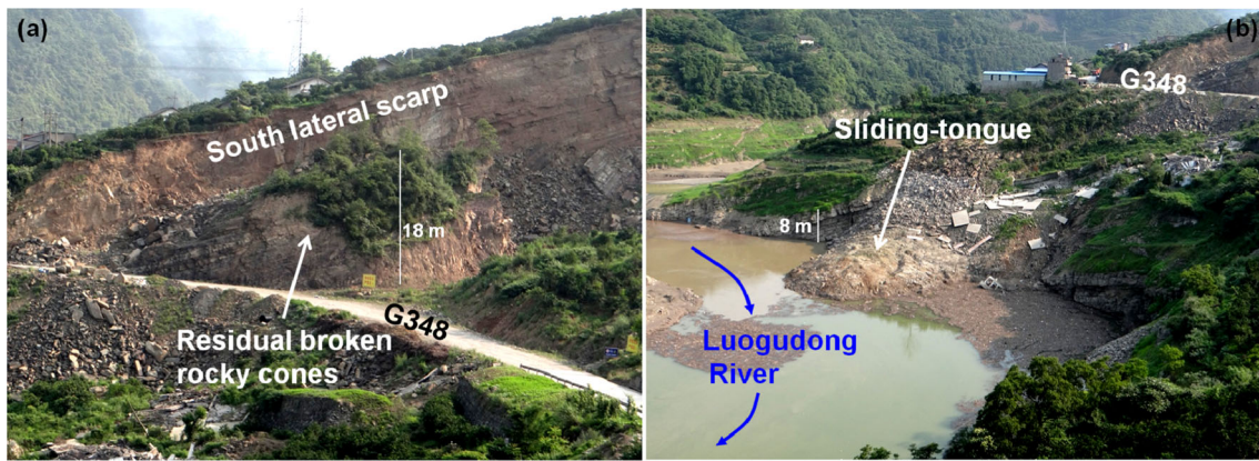
Fig. 15 Photos of the rear and front parts of the southern rocky sliding mass. a The residual broken rocky cones above G348 and b sliding tongue on the front riverbed
