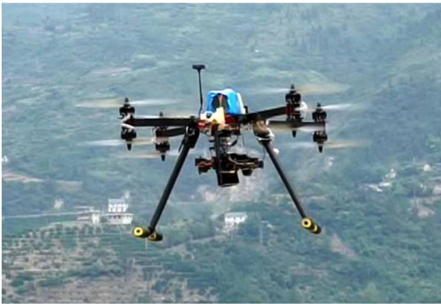
Fig. 5 The micro-UAV that was used to capture photos and generate georeferenced orthomosaic and DSM of the post-landslide area on June 19, 2015
