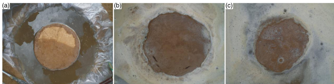
Fig. 11 Images of the process of loess disintegration
