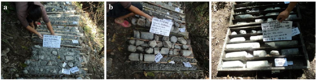
Fig. 3 Cores drilled from boreholes of three strata at Huangjiazhai Tunnel: (a) gravelly soil; (b) heavily weathered shale; and (c) moderately weathered shale
