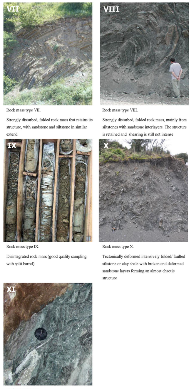
Fig. 6 Examples of rock mass types (types VII to XI) of flysch corresponding to descriptions in Fig. 4
