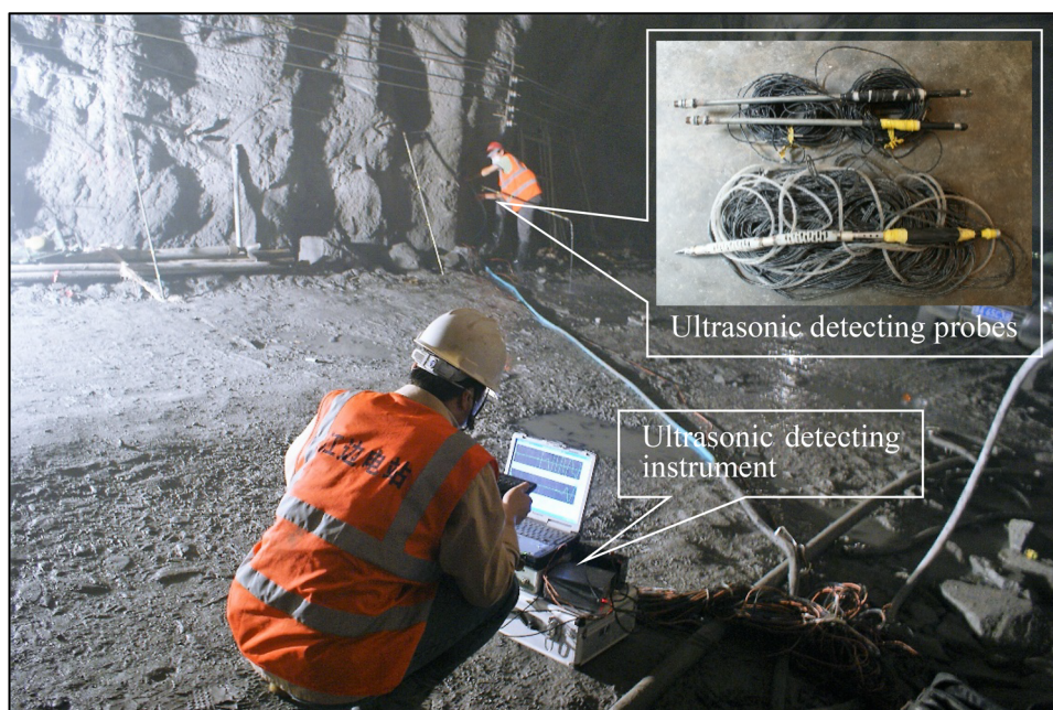
Fig. 7 Rock-mass integrity index determined by ultrasonic detecting instrument
