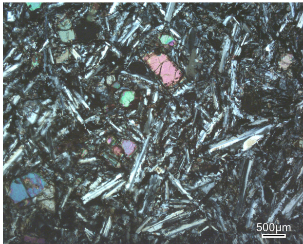
Fig. 2 Thin section (crossed nicols) from basalt quarried at “Su Inzale”
