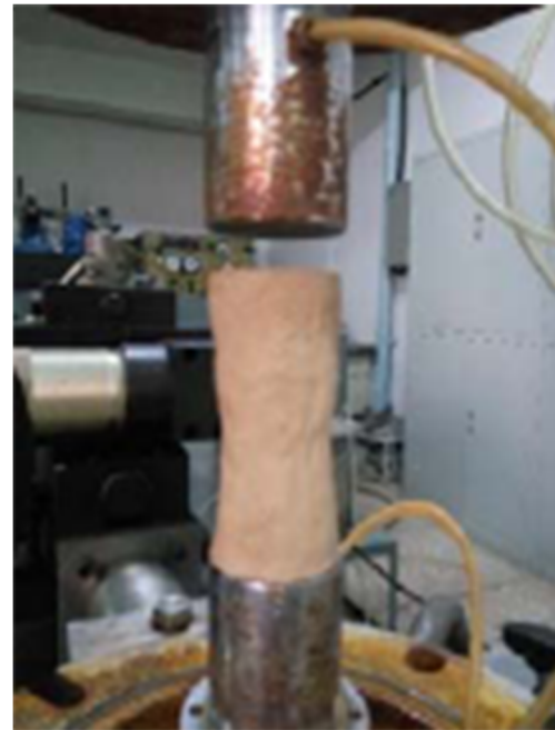
Fig. 5 Typical tensile failure
