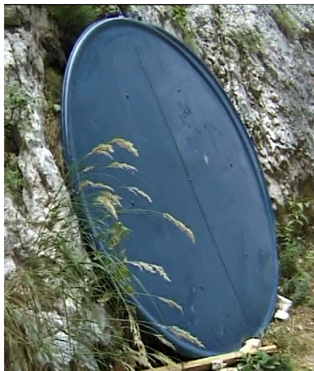
Fig. 2 Sheet metal jack (example from the investigation works at the Komarnica Dam, Montenegro)
