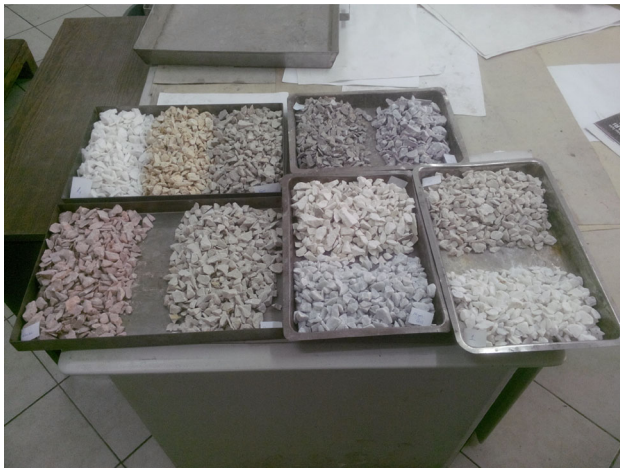
Fig. 3 Some of the crushed rock samples in the size range of 19.00–9.52 mm
