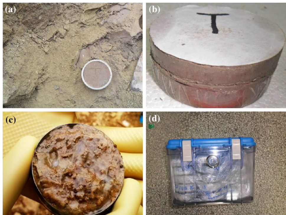
Fig. 1 Collection process of the mudded weak interlayer specimens
