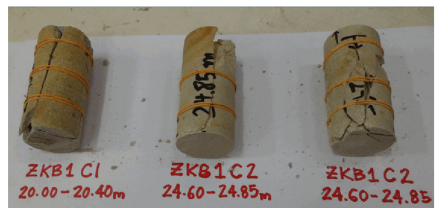
Fig. 5 Fracture planes in failed rock samples after performing UCS tests
