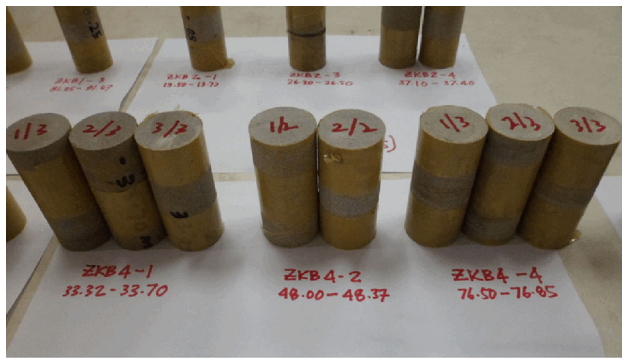
Fig. 4 Some of the cylindrical core samples prior to UCS tests
