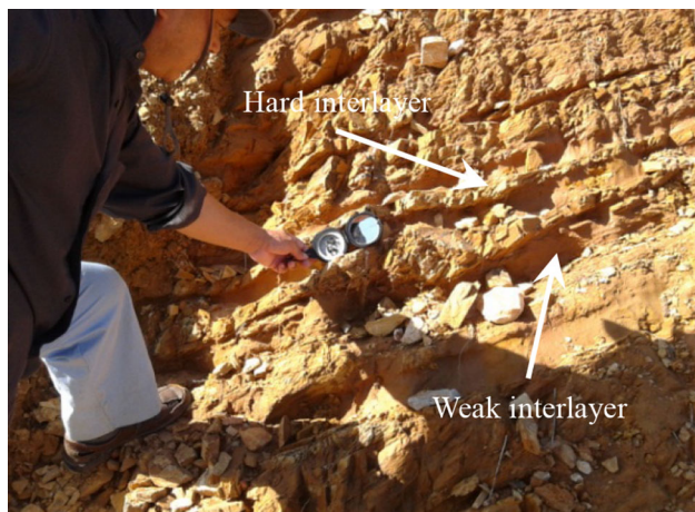
Fig. 2 Soft and hard interbedded rock
