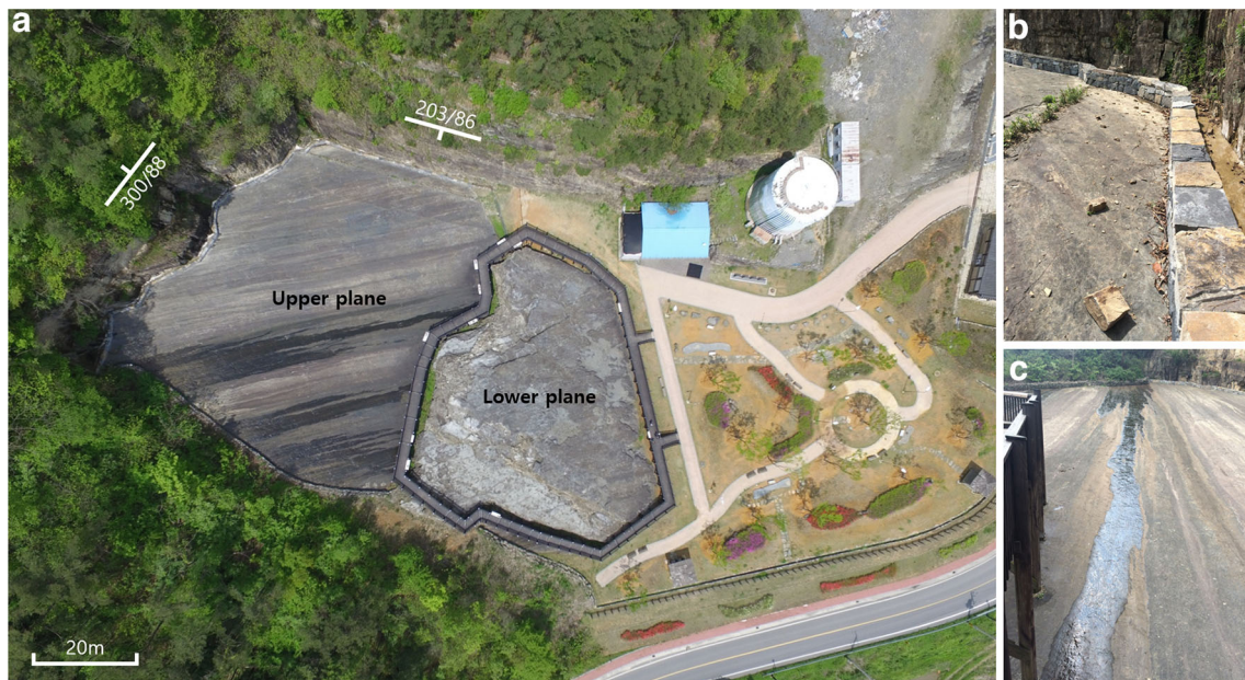
Fig. 3 Engineering geological properties of the site. a The site is surrounded by northern and western slopes which have a nearly 90° inclination. b Rockfall was observed, which can damage the tracksite
