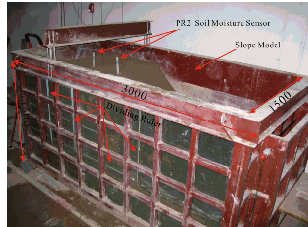
Fig. 2 Photograph of the model test chamber (unit: cm)
