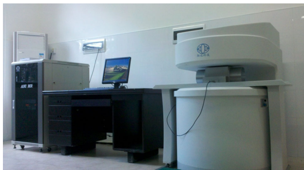
Fig. 1 AniMR-150 NMR imaging system
