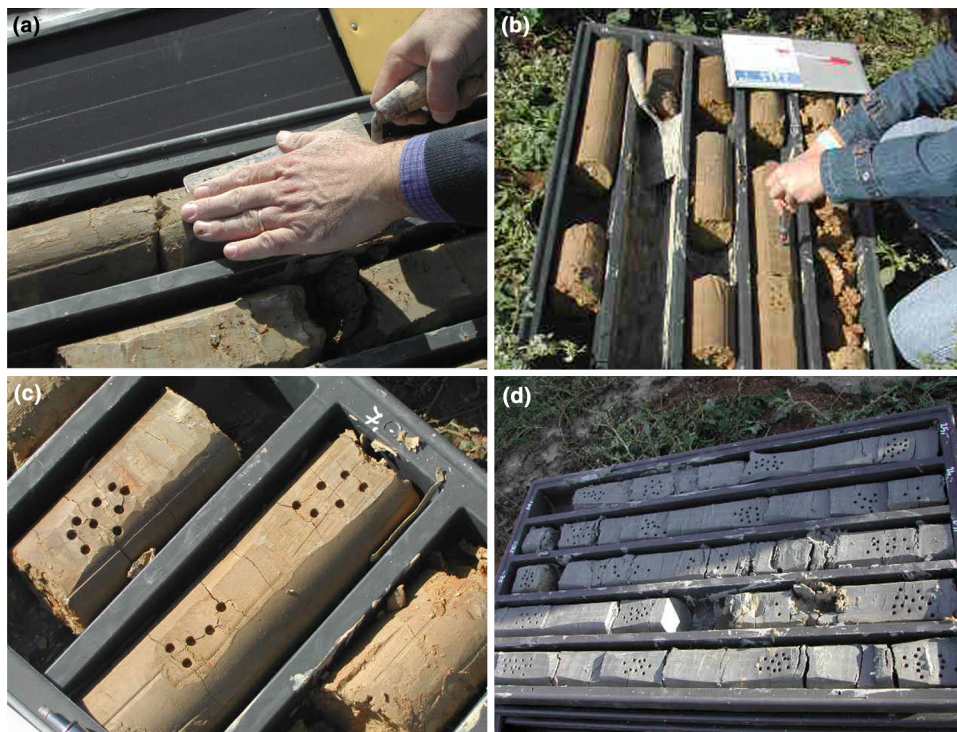
Fig. 2 Data collection. a Removal of the disturbed surficial portion of samples. b Execution of measurement on the collected samples. c, d Some samples subjected to the measurements
