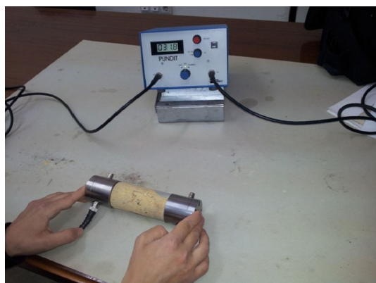
Fig. 9 Ultrasonic velocity test
