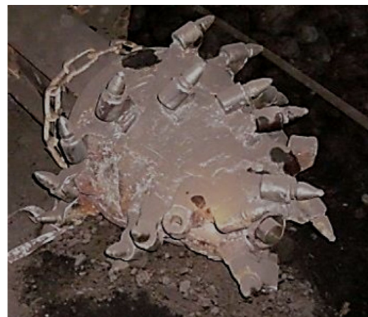
Fig. 4 The cutter head of Dosco Mk-2B roadheader
