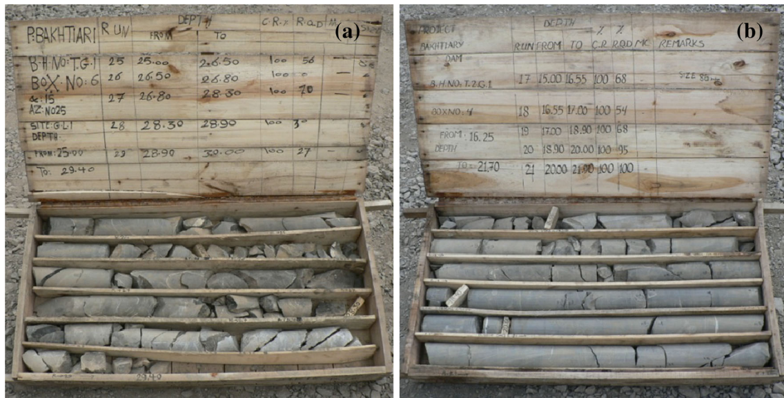
Fig. 5 Sample cores of the trial grouting boreholes in a the left and b the right abutments
