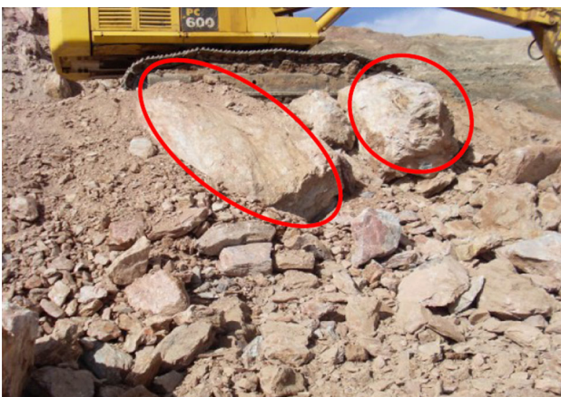
Fig. 3 Boulders resulting from blasting operations at the Anguran mine
