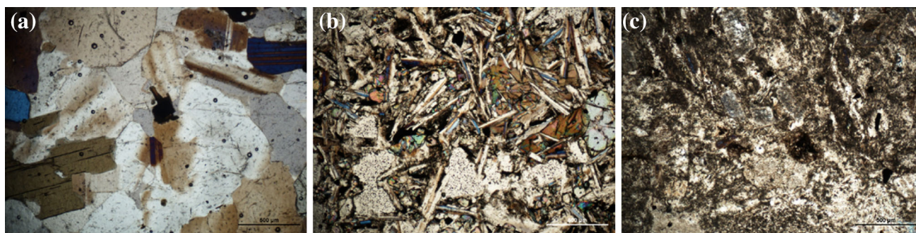
Fig. 2 Thin section microscopy images of rock specimens with polars crossed ( \times 5 ). a Diorite was coarse-grained rock consisting of plagioclase, olivine, micas, quartz, and microcline. b Basalt consisted mainly of needle-shaped plagioclase, olivine, quartz, micas, and
