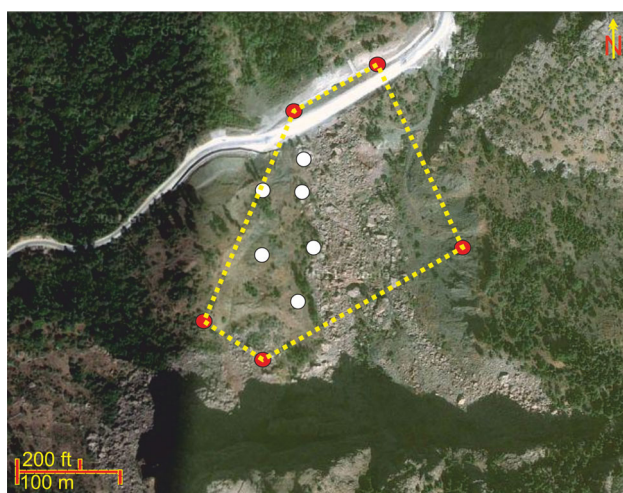
Fig. 5 Position of terrestrial laser scanning stations and locations of ground control points
