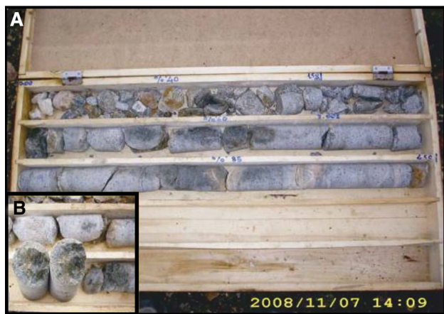
Fig. 2 a Core box and b typical rock core with joints used in the shear tests
