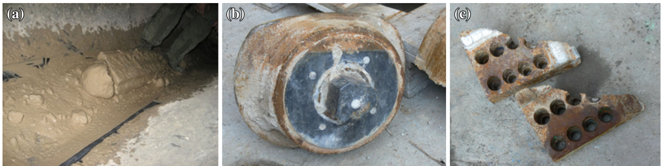
Fig. 13 Damage of TBM parts and excessive wear of tools. a Breakage of cutter tools due to boulder interaction, b flat wear of cutter disc, c wear of bucket tool
