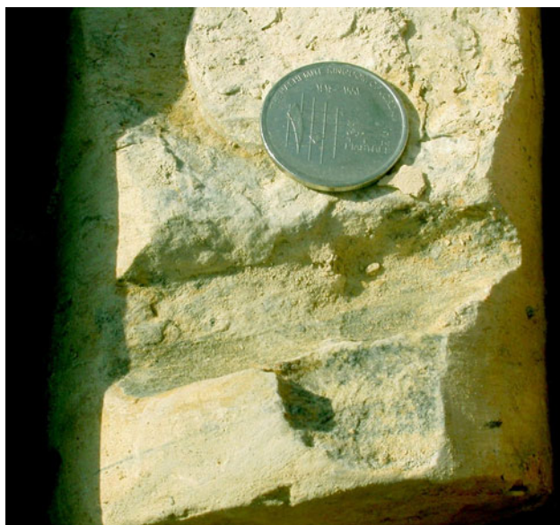
Fig. 10 Linear karst channel in NX core, Wing Section, right abutment
