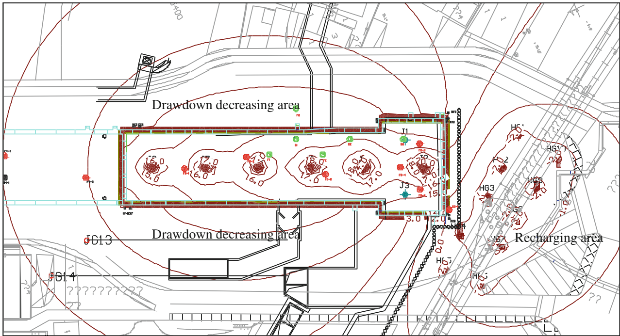
Fig. 20 Water table contour of layer \mathcal{D}_2 under pumping and recharging condition (in plane)
