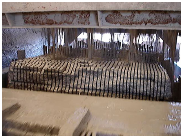
Fig. 6 Distribution system of the abrasive mixture in the sawing of siliceous dimension stones
