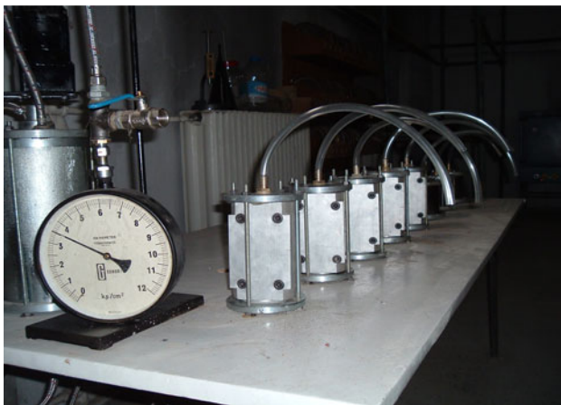
Fig. 3 Grouting test setup
