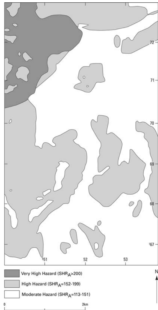
Fig. 7 Subsidence hazard assessment for deneholes, Dartford, UK. Original scale 1:25000 (from Edmonds et al. 1987)
