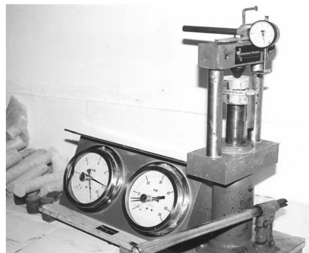
Fig. 3 Indentation testing using point load apparatus
