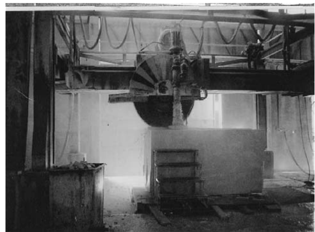
Fig. 1 A block cutting machine trimming the surface of the stone block
