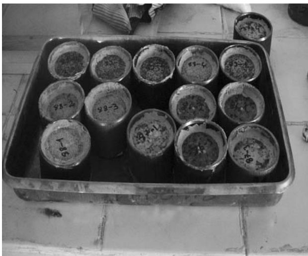
Fig. 2 Cemented samples in the steel frames
