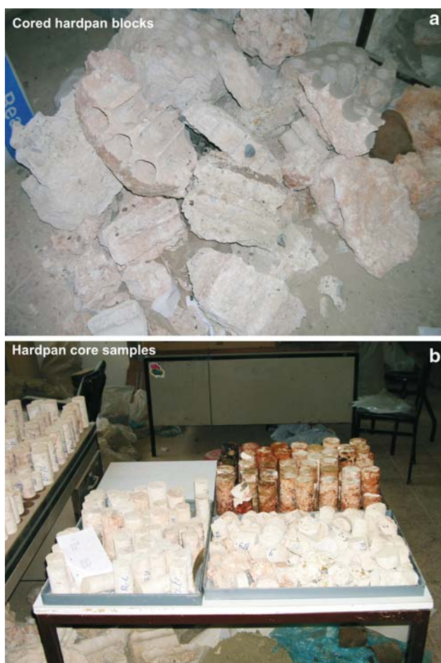
Fig. 4 a Cored caliche blocks, b NX and BX size caliche core samples
